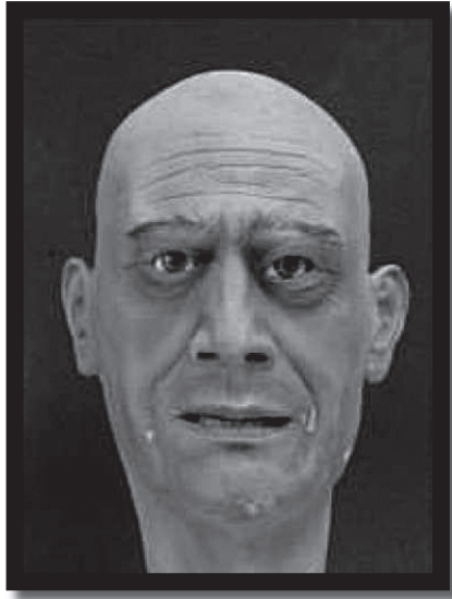
Fig. 2. A previous version of the humanoid robot. ROMAN™ (ROMAN = RObot huMan interAction machiNe) with human-like silicon skin.
