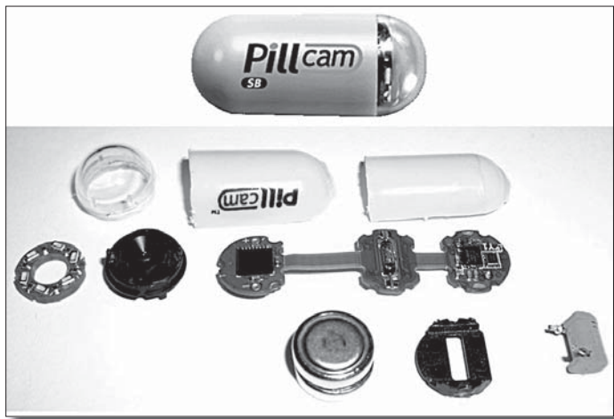
Figure 5: PillCam SB (Given Imaging Inc., Israel) and its components (shell cut into half).
