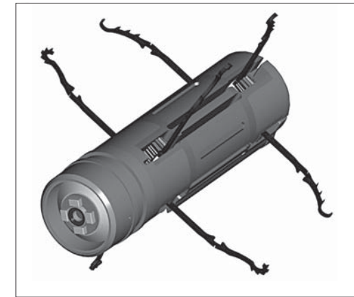
Figure 6: Legged capsule prototype for locomotion in the gastrointestinal tract (Source: CRIM lab, Scuola Superiore Sant'Anna, Pisa, Italy).
